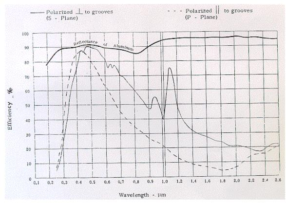
**Note:** Efficiency curves shown are relative (not absolute), are only representative, and can vary significantly depending on use geometry and measurement technique. Two masters with the same catalog number may have different efficiency curves. The uncertainty band on the data in the above relative efficiency curve(s) is  $\pm$ - three percentage points. Maximum Ruled Area is expressed as L x W, where L is the length of the grooves and W is the ruled width.
