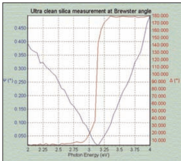
Measurement on ultra-clean silica at the Brewster angle
